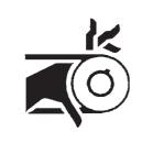
The presence of dangerous mechanims inside the machine can cause serious injuries. Respect all safety instructions before doing any work on the machine. Replace protective casings after doing any work.
